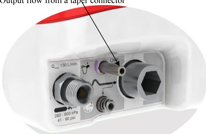
Fig. 2u: CPAP & Flow Connector
