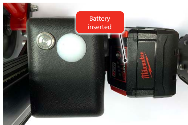
Battery fitted correctly
