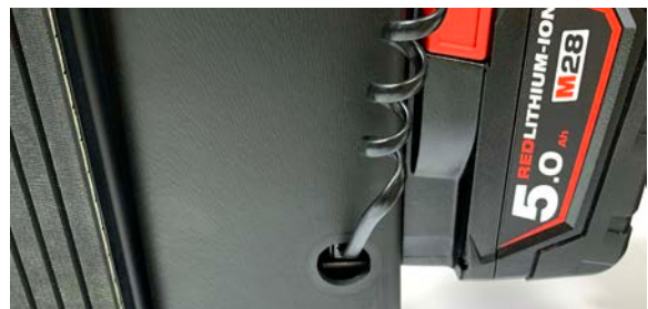
Figure 13 - Connecting the cable to the motor housing
