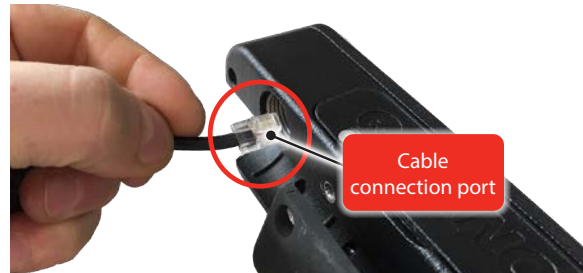
Figure 11 - Connecting the cable to the connector port
