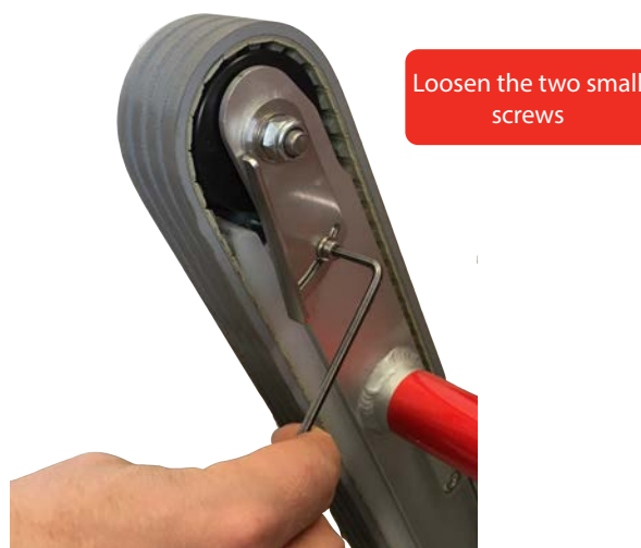
Figure 5 - Loosen the two small screws
