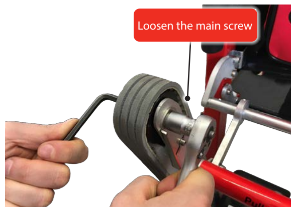
Figure 4 - Loosen the main screw
