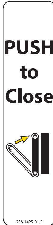
Label showing how to close the track carriage
