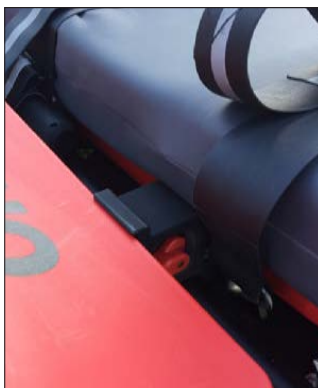
Ensure Scoop fins are positioned under the holding plates
