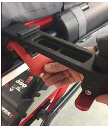
Attaching fixing bracket to siderail interface
