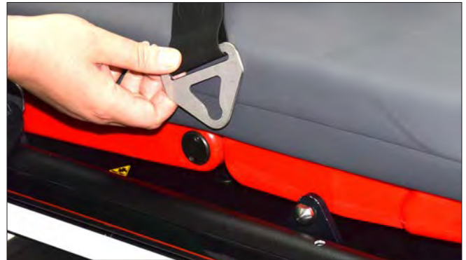
Strap tang with fixing hole
