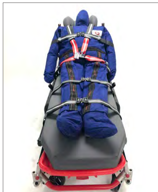
4-point harness,chest strap and leg straps applied
