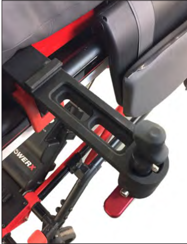
Fixing bracket lift-up locking arm
