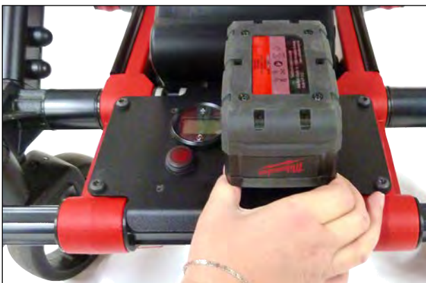
Removing battery pack
