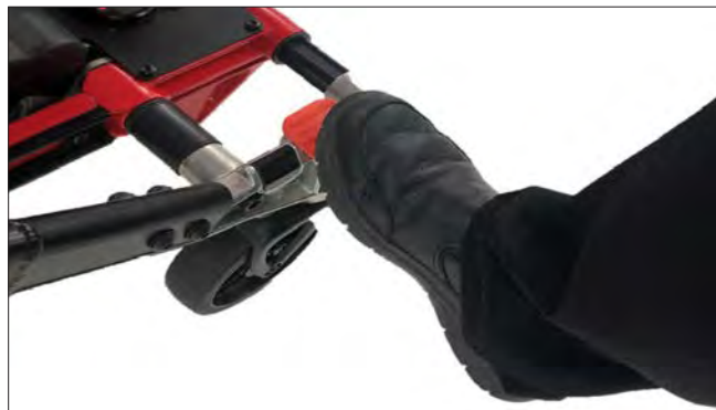
Disengaging wheel brake push forward and down
