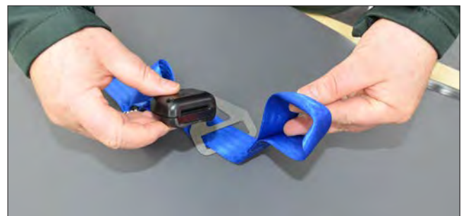
Loop strap and tang attached to PediMate fixing strap
