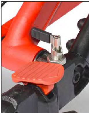
Directional wheel lock with manual-operated lever. Lever pointing inwards denotes lock disengaged
