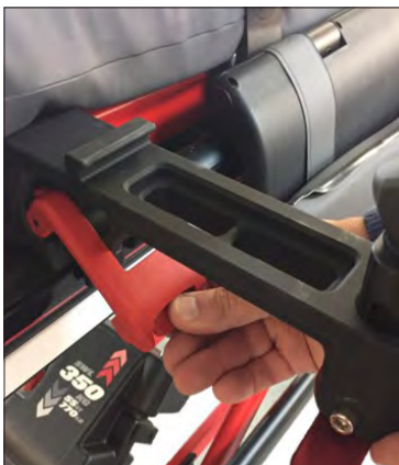
Attaching fixing bracket to siderail interface
