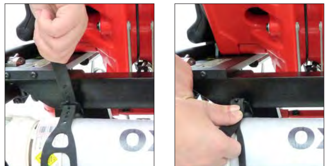
Securing straps on O2 holder
