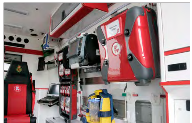
Ferno's IPTS iNTRAXX wall track bracket system
