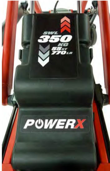
Safety Instruction: Safe Working Load label on actuator cover
