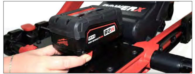
Removing battery pack
