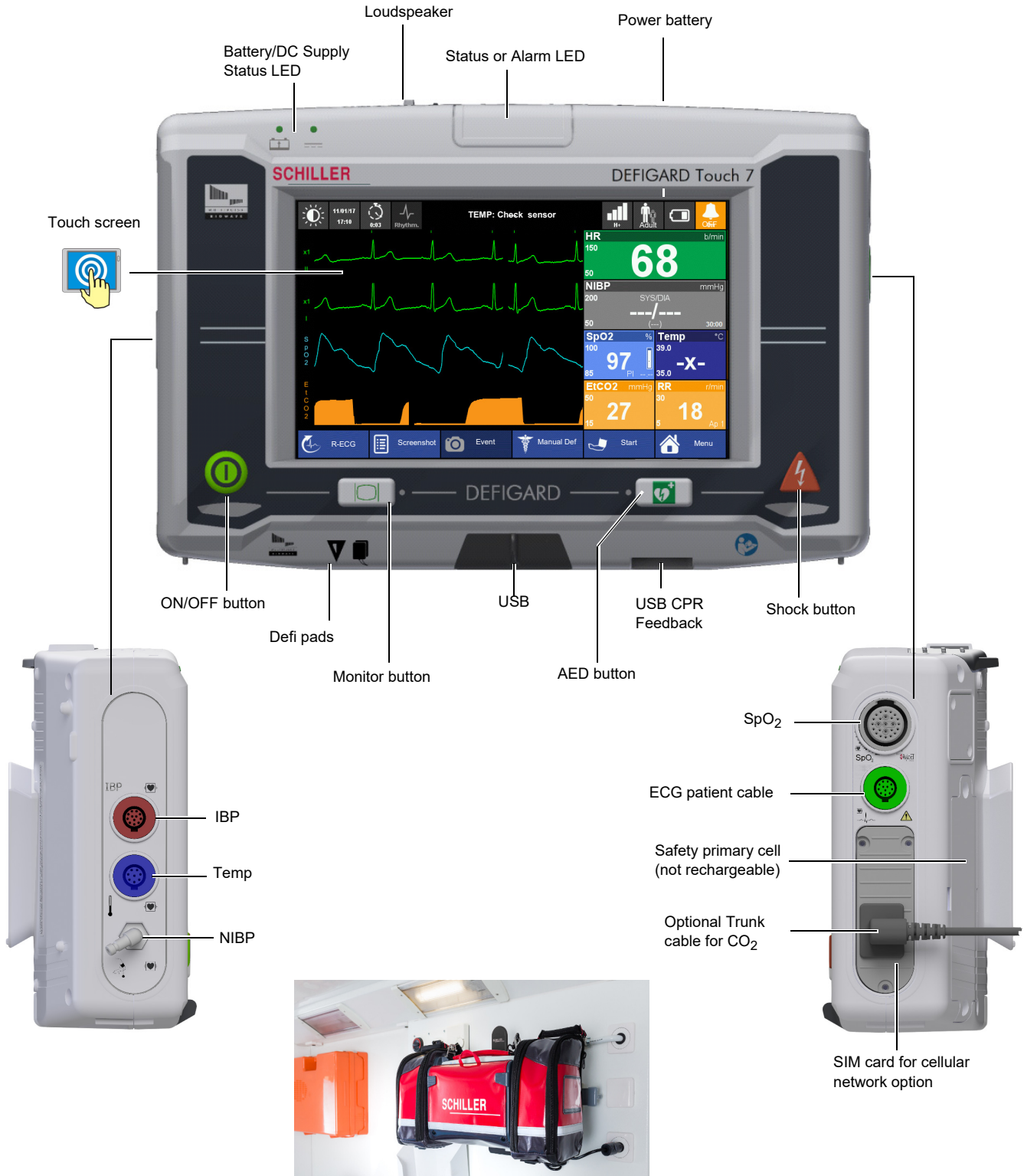
Fig. 2.1 Front panel and device controls
