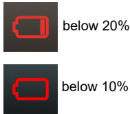
Fig. 3.3 Battery low indication
